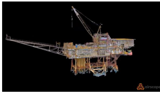
Screenshot of the Kingfish A 3D model created using imagery captured by an Airscope Industries drone
