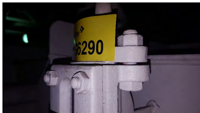
Photo 64 G6290 3rd Deck Engine Room, Turbine, Lube Oil Gravity Tank Level Sight Glass Flange – Gasket (Chrysotile)
