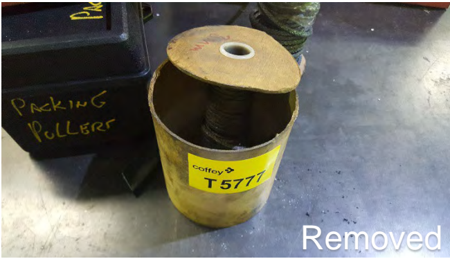
Photo 43 T5777 3rd Deck - Workshop, Bulkhead penetration insulation Cabinet, Second Shelf Labelled (General Purpose Temperature) – Bulkhead penetration insulation 'No Brand' (Chrysotile)
