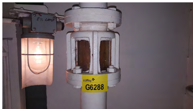
Photo 62 G6288 3rd Deck - Engine Room, Turbine, Lube Oil Gravity Tank Over Flow Sight Glass Flange - Gasket (UMF)
