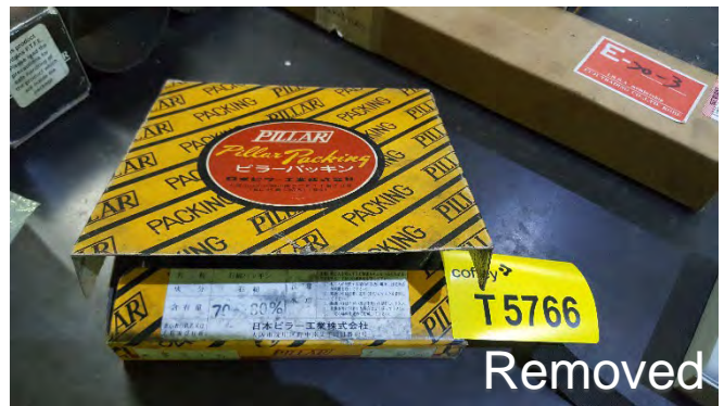
Photo 40 T5766 3rd Deck - Workshop Bulkhead penetration insulation Cabinet, Top Shelf Labelled (Steam Bulkhead penetration insulation Shelf)– Bulkhead penetration insulation 'Pillar' (Chrysotile)
