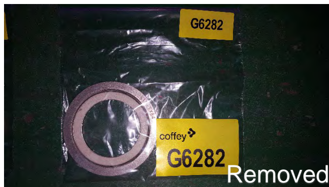
Photo 86 G6282 2nd Deck Storage Area, BF2 – Spiral Wound Gasket, Sealing Element (Cream)'Vortex 20x32x63 CT' (Chrysotile)
