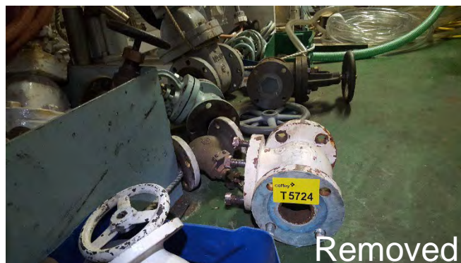
Photo 26 T5724 3rd Deck Workshop Mezzanine, Starboard, Fore, Adjacent Handrail, Stored Items (In Blue Plastic Tub) – Gasket Material Adhered to Flange (UMF)
