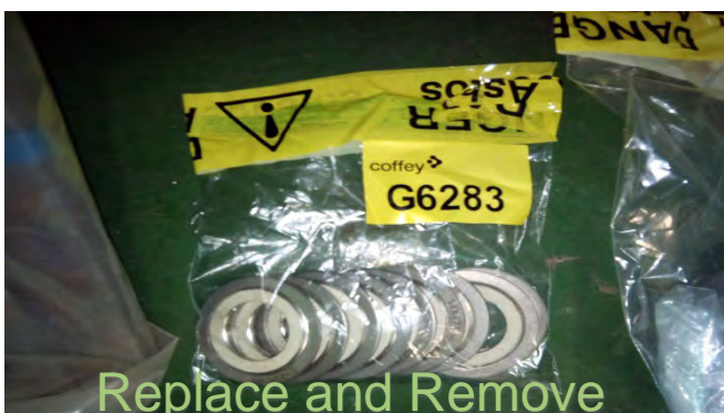
Photo 87 G6283 2nd Deck Storage Area, Contained for Removal – Spiral Wound Gasket, Sealing Element (White) 'C-20K-20' (Chrysotile)
