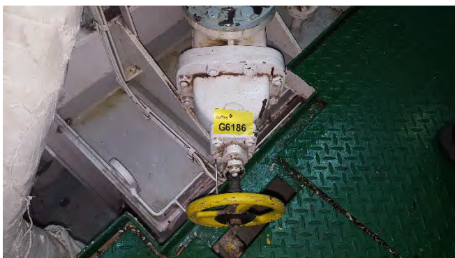
Photo 19 G6186 4 th Deck - Purifier Room, Lube Oil Purifier No.2, Sludge Dump Valve – Gasket (UMF)
