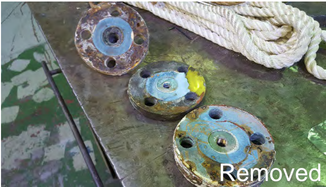
Photo 43 T5777 3rd Deck - Workshop, Bulkhead penetration insulation Cabinet, Second Shelf Labelled (General Purpose Temperature) – Bulkhead penetration insulation 'No Brand' (Chrysotile)
