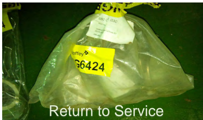
Photo 146 G6424 2nd Deck Storage Area, Contained for Reassurance Return to Drawer BG3, Gasket, Gasket (Ring) [680.01.01.030 (No Asbestos Detected)
