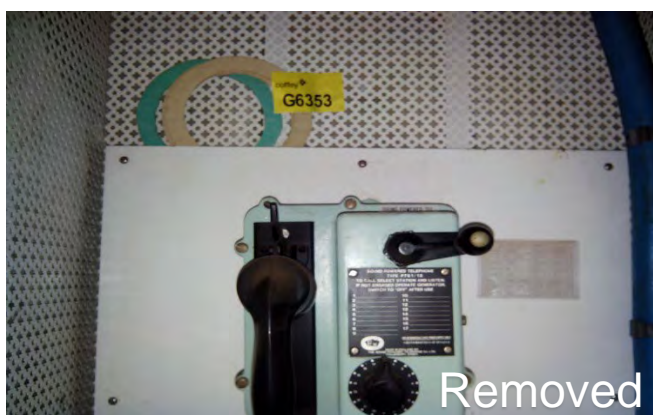
Photo 103 G6343 Upper Deck - Dry Chemical Unit Room, Aft, Outlet Storage, Under Manifold – Gasket (Chrysotile)
