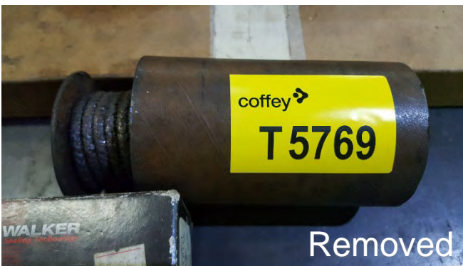
Photo 41 T5769 3rd Deck Workshop Bulkhead penetration insulation Cabinet, Top Shelf Labelled (Steam Bulkhead penetration insulation Shelf) – Bulkhead penetration insulation 'No Brand' (Chrysotile)
