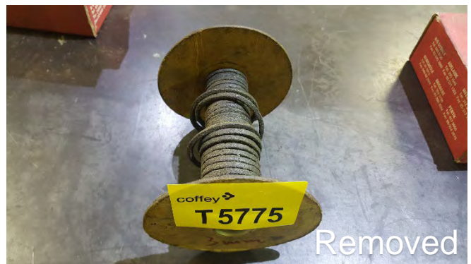
Photo 42 T5775 3rd Deck - Workshop, Bulkhead penetration insulation Cabinet, Second Shelf Labelled (General Purpose Temperature) – Bulkhead penetration insulation 'No Brand' (Chrysotile)
