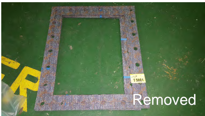
Photo 83 T5861 2nd Deck Storage Area, Contained for Removal – Gasket Loose 'Valqua 1755' (Orange Font with Black Backing and White Specks) (Chrysotile)
