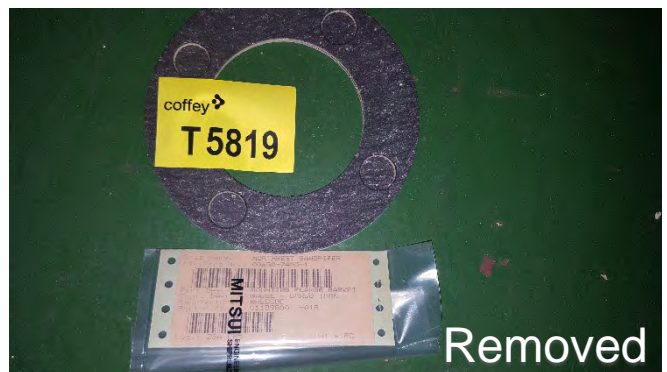
Photo 72 T5819 2nd Deck - Storage Area, Drawer CB5, (Labelled Cargo Tank Gauges) - Gasket Loose 'No Brand' Black with White Specks (Chrysotile)
