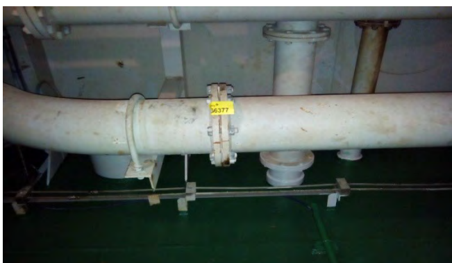
Photo 113 G6377 Upper Deck Pipe Passage Starboard, IG Pipe Flange (Aft) - Gasket (Chrysotile)
