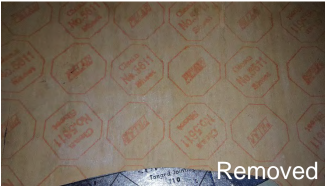
Photo 37 Refer to T5749 3rd Deck - Workshop, Bulkhead penetration insulation Draws, Fourth Draw (Labelled Supergraph) – Gasket 'Pillar Clean Sheet No. 5611' (Presumed Positive)
