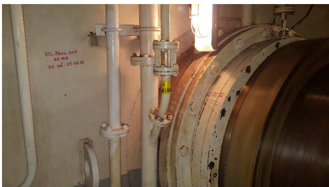
Photo 7 G6164 Lower Deck - Engine Room, Aft Midship, Sight Glass, Stern Tube to Lube Oil Overflow- Gasket (UMF)
