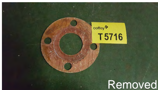
Photo 24 T5716 3 rd Deck - Workshop Mezzanine, Starboard, Fore, Stored Item – Gasket Loose t (Pink, Black Font, Tombo 1100) (Chrysotile)
