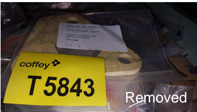
Photo 77 T5843 2nd Deck Storage Area, Drawer, AE5 Diesel Generator – Gasket Loose 'Valqua' (Beige Backing Black Print, 350.01.01.G50) (UMF)
