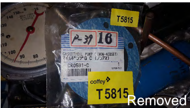
Photo 71 T5815 2nd Deck Storage Area, Drawer CC2 (Labelled Refrigerator Tools and Fittings) Gasket Loose 'YMcO' CR0591-C (Blue) (Chrysotile)
