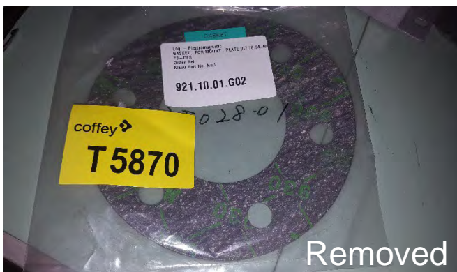
Photo 133 T5870 F Deck - No.2 Equipment Room, Drawer DE8 – Gasket Loose 'Valqua 930' Electro-Magnetic Mount 921.10.01.G02 (Chrysotile)
