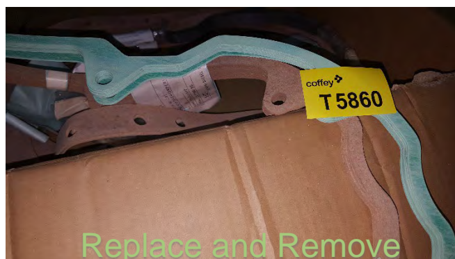
Photo 82 T5860 2nd Deck - Storage Area, Above BD5 Cabinet – Gasket Loose (No Brand) Green with Yellow Specks 350.01.01.073 (UMF)
