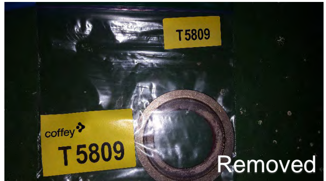
Photo 70 T5809 2nd Deck - Storage Area, Drawer CC1 (Labelled Spare Spiral Wound Gaskets) Throughout - Gasket Loose Spiral Wound Graphite/Cream Sealing Element, Valqua SHAS 304 (Chrysotile)
