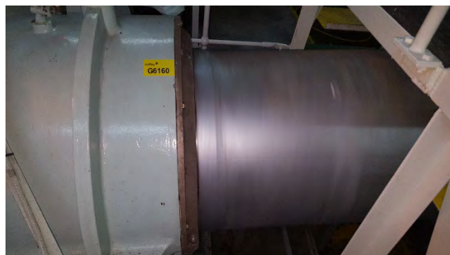
Photo 8 G6160 Lower Deck Engine Room, FWD Upper Face, Tail shaft Bearing Cover, Upper Face – Gasket (UMF)
