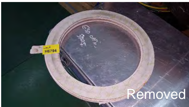
Photo 95 G6794 Upper Deck, No1 Cargo Room on Storage Rack, Gasket Loose "Valqua 1501" Grey Background Green Font (x14) (Chrysotile)
