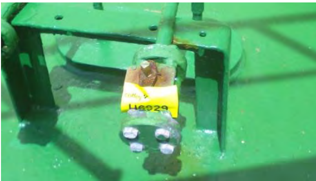
Photo 135 H6929 Upper Deck, No.2 Cargo Hold N2 Blanked Sampling Point, Gasket (Chrysotile)
