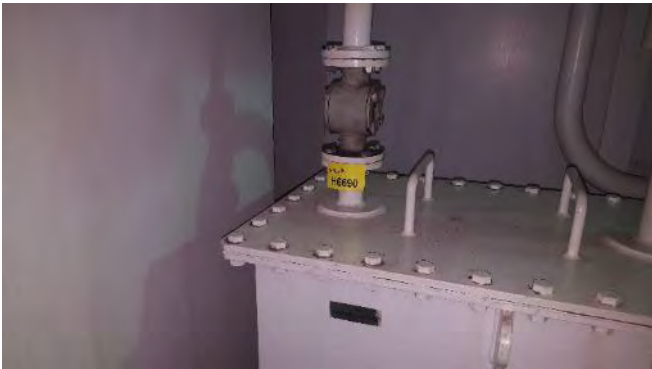
Photo 53 G6690 3rd Deck, Steering Flat, Overflow Tank Filling Glass Flange, Gasket (Chrysotile)
