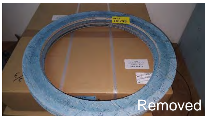
Photo 94 G6793 Upper Deck, No1 Cargo Room on Storage Rack, Gasket Loose "Tombo 1000" Blue Background Black Font (x16) (Chrysotile)
