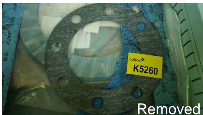
Photo 160 K5260 2nd Deck, 2SA, BJ3 708.10.01.024 Manoeuvring Valves, Gasket "Valqua 1500" Black Backing with Green Font (Chrysotile)
