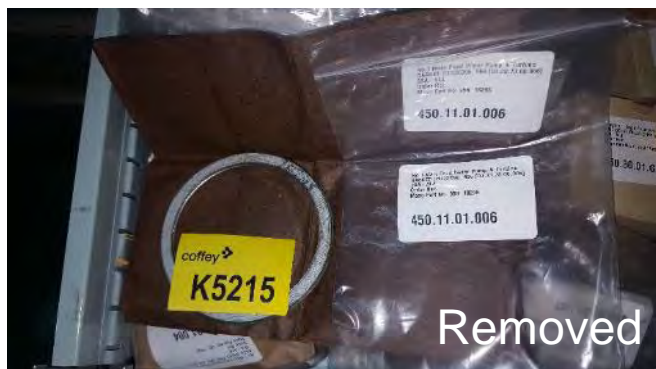
Photo 152 K5215 2nd Deck, 2SA, AL4 45011.01G4, Spiral Wound Gasket (White Sealing Element) Branded 'Coffin' (Chrysotile)
