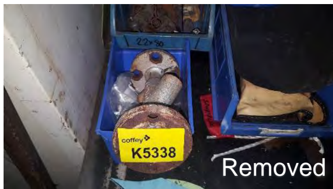
Photo 188 K5338 3rd Deck, Workshop, Gasket Drawer Bench Top, Stored Valve, Gasket Adhered to Valve (Chrysotile)
