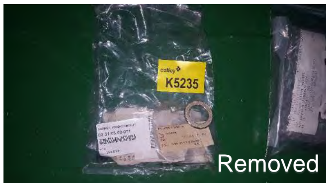
Photo 156 K5235 2nd Deck, 2SA, BE3 709.71.01.071, Main Steam System Traps Gasket (Chrysotile)
