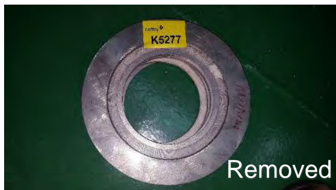
Photo 172 K5277 2nd Deck, 2SA, BJ2, Spiral Wound Gaskets Large Size (158x173x203 JPI900-6 (Chrysotile)
