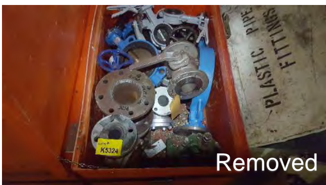
Photo 183 K5324 2nd Deck, Workshop Loft, Small Red Metal Box, Gasket Adhered to Silver Valve (Chrysotile)
