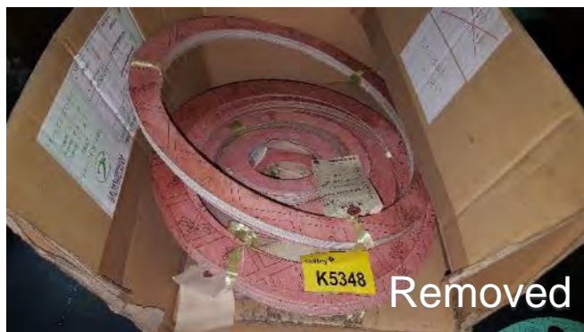
Photo 190 K5348 3rd Deck, Workshop, Storage Rack, Gaskets Loose "Tombo 1000" Tan Backing Black Font (Chrysotile)
