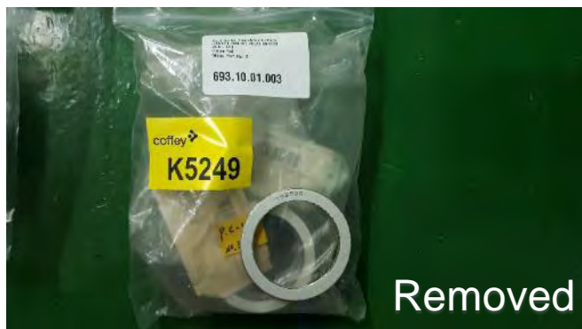
Photo 158 K5249 2nd Deck, 2SA, BF1 693.10.01.003 Soot Blower, Spiral Wound Gasket (Chrysotile)
