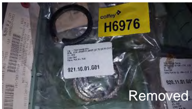
Photo 148 H6976 F Deck, No.2 Equipment Room, F3 DE8 921. 10.01.G01, Electromagnetic Seal, Packing Gland (Chrysotile)
