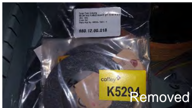
Photo 174 K5294 2nd Deck, 2SA, CB5 Cargo Tank Gauging 880.12.00.018, Gasket (Black with White Speckles) (Chrysotile)
