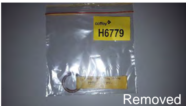
Photo 89 H6779 2nd Deck, Control Room, Starboard Cupboard to Wooden Cabinet, Small Spiral Wound Gasket (White Sealing Element) '1 Mpa Steam Trap Valves (Chrysotile)
