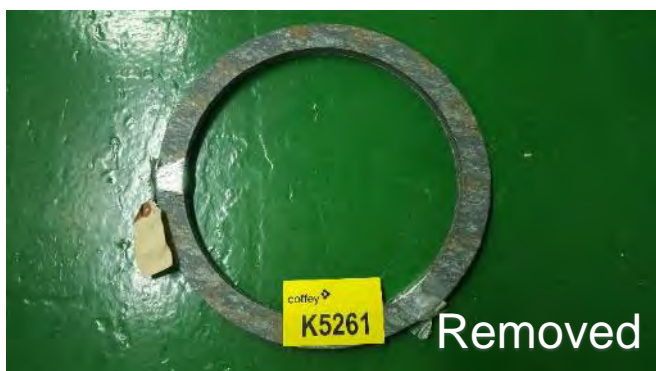
Photo 161 K5261 2nd Deck, 2SA, BJ2, Gasket "Valqua" (Chrysotile)
