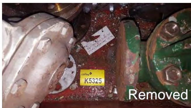
Photo 184 K5325 2nd Deck, Workshop Loft, Small Red Metal Box, Debris (Mixed) (Chrysotile)
