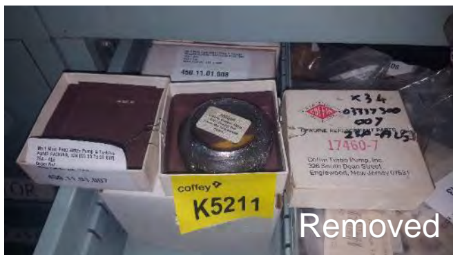
Photo 151 K5211 2nd Deck, 2SA, AL5 450. 11.01.007 Pump Packing, Packing 'Coffin' (Chrysotile)
