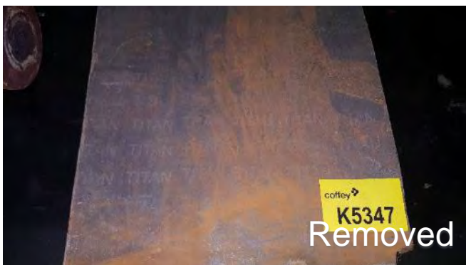
Photo 189 K5347 3rd Deck, Workshop, Storage Rack, Gasket Sheet "Titan" (Grey Backing Silver Font) (Chrysotile)
