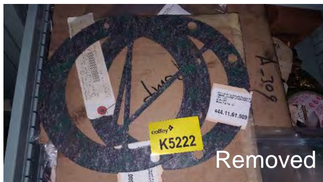
Photo 154 K5222 2nd Deck, 2SA, AE3 444.11.01.009 Main Condenser Vacuum Pump Nash International, Gasket "Valqua 1500" Black Backing with Green Font (Chrysotile)
