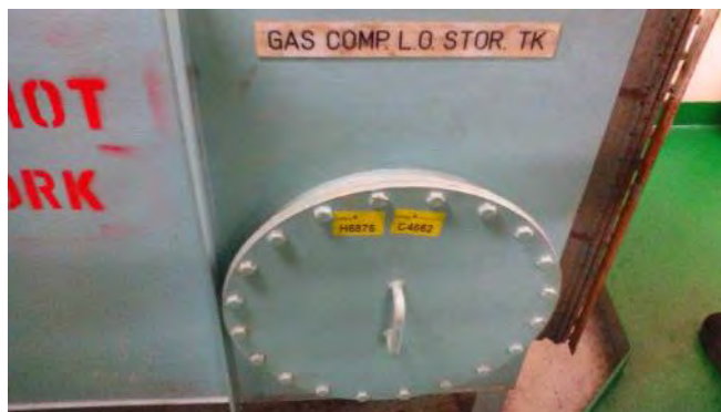
Photo 118 H6876 Upper Deck, Cargo Motor Room, Gas Compressor L.O. Storage Tank Manhole Cover, Gasket (Chrysotile)
