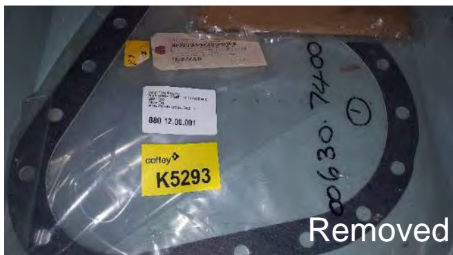
Photo 173 K5293 2nd Deck, 2SA, CB5 Cargo Tank Gauging 880.12.00.001, Gasket Loose "Permanite G" (Black Backing with White Speckles and Blue Font" (Chrysotile)
