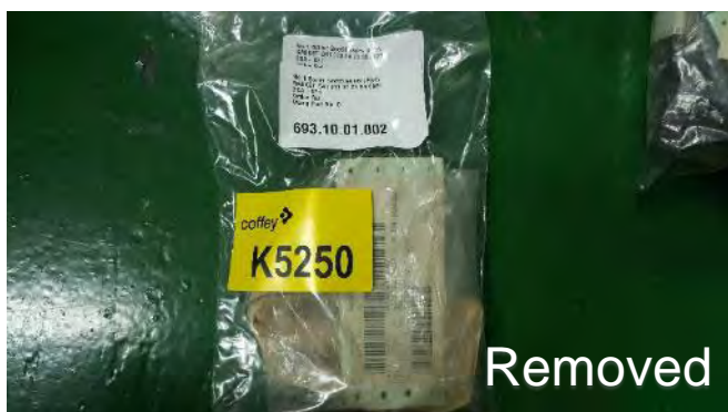
Photo 159 K5250 2nd Deck, 2SA, BF1 693.10.01.002 Soot Blower, Gasket Metal (Chrysotile)
