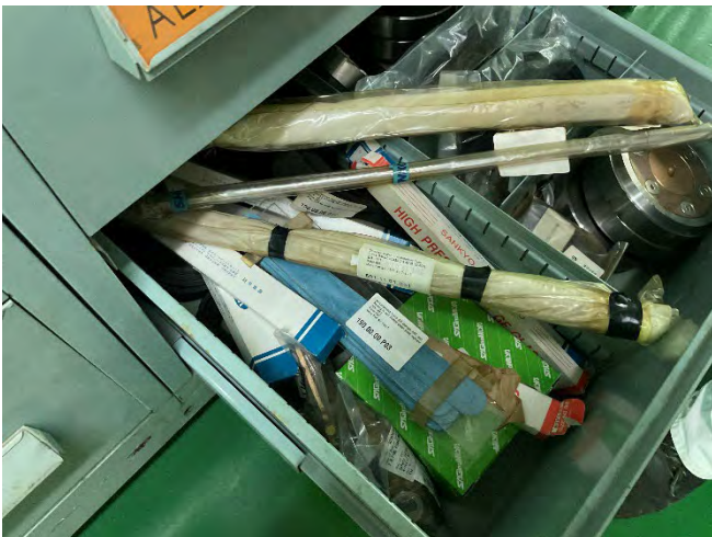
Photo 95 ZA21841 2nd Deck 2as Drawer AH2 - Spare Forward fire pump gasket (Chrysotile)
