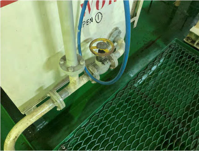
Photo 41 Q5369 Focsle store -starboard Aft - hyd trans P/P suction Gasket to hyd trans P/P suction
