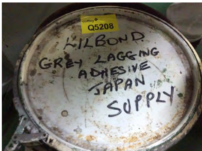
Photo 31 Q5208 2nd deck - 2sa - hc1 drawer Drum of Kilbond grey lagging adhesive
