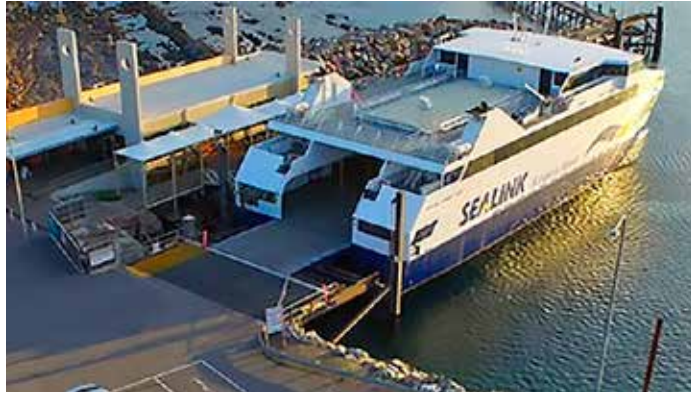
Sealion 2000 is 800 gross tons, 49 m long. She was built at Jervoise Bay WA, in 1998
